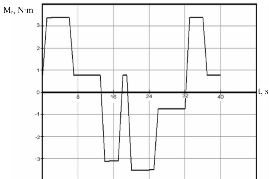
Figure 5. Diagram of rotational moment change on the transmission shaft of manipulator drive obtained via calculation
