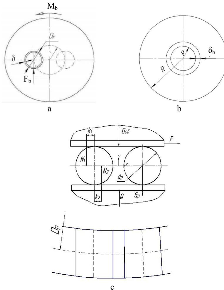
**Figure 2.** Computational models for definition of components of static moment of resistance to moving bearing body caused by force action: *a* - metal sinterskin cutting; *b* - force of sliding friction between contact surfaces of refractory plates during their relative motion; *c* - rolling friction in bearing assembly
