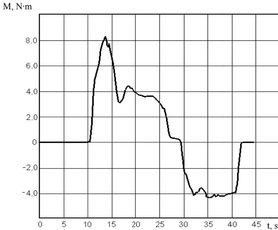
Figure 3. Signal type registered at control of rotational moment caused by drive of hinged gate physical analogue
