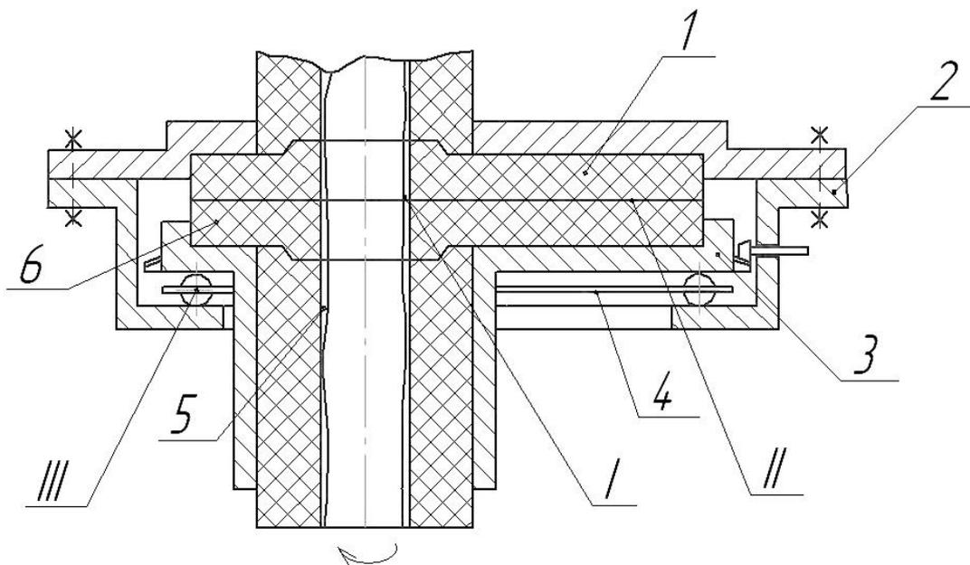
**Figure 1.** Kinematic scheme of hinged gate with identification of zones, in which the components of static moment of resistance to moving bearing body act: 1 - refractory plate, 2 - gate body, 3 - moving bearing body, 4 - rolling-contact bearing, 5 - metal sinterskin, 6 - refractory plate
