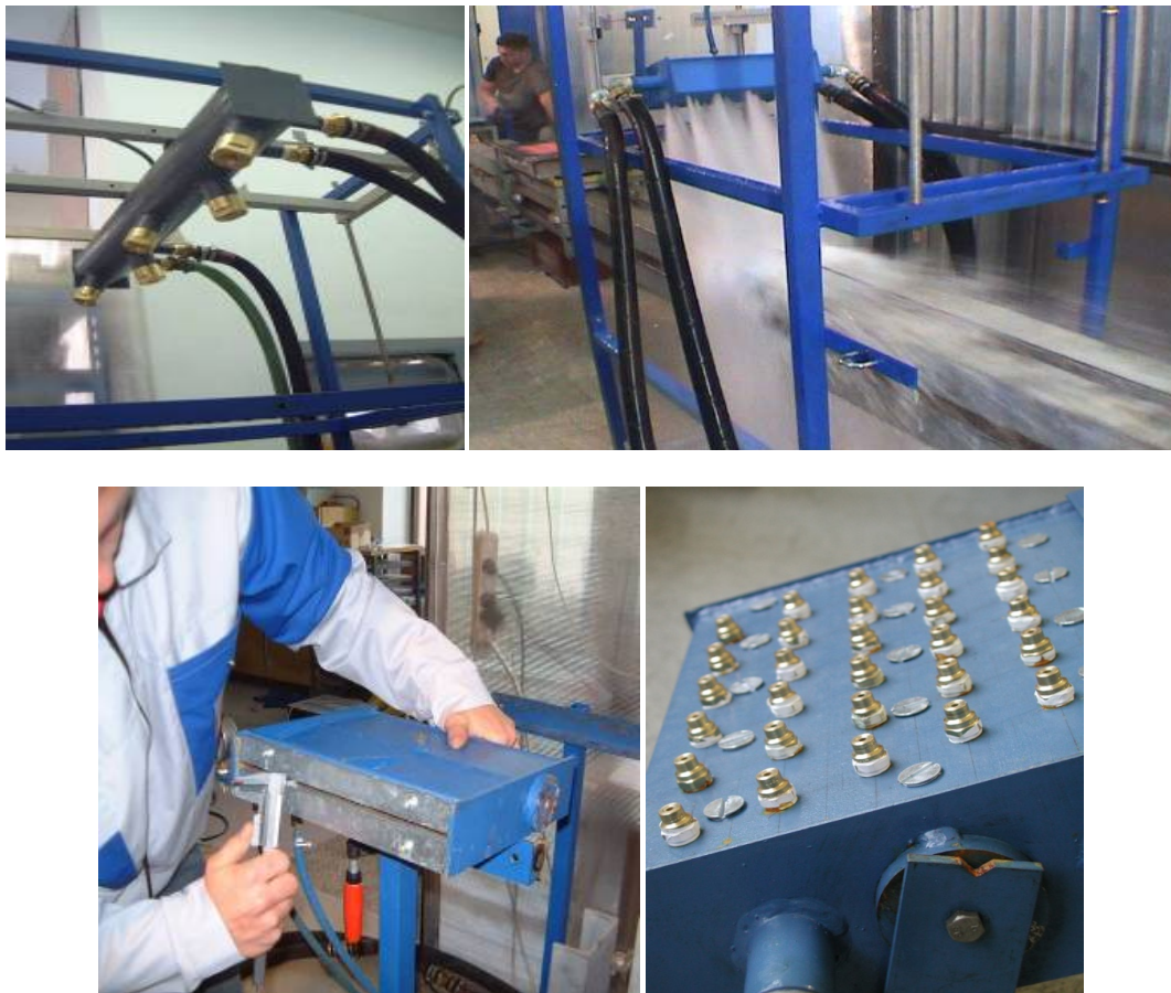
Figure 2. Various types of cooling headers (full cone nozzles, drilled holes, adjustable slit, cluster of solid jet nozzles)
