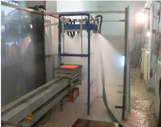
Figure 1. Linear laboratory stand with test plate moving under group of full cone nozzles
