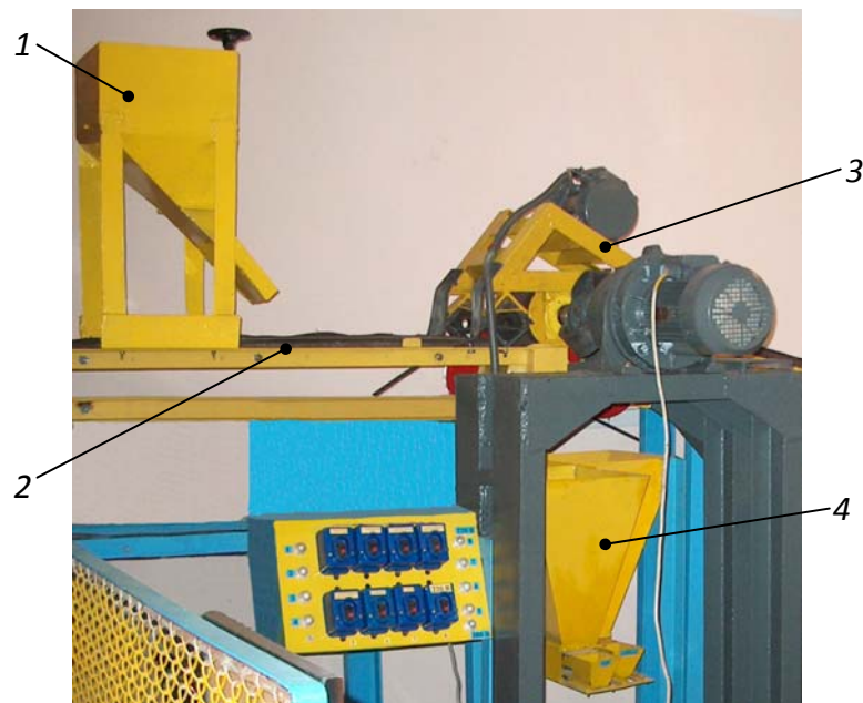
Figure 1. Laboratory-scale plant of sinter burden repressing; 1 - charging hopper; 2 - conveyor; 3 - represser; 4 - receiving hopper
