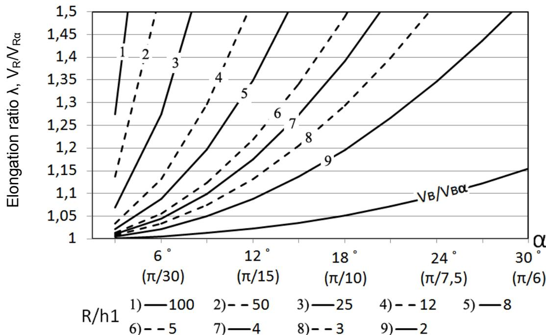
**Figure 1.** Dependence of elongation ratio  $\lambda$  and ratio  $V_R/V_{R\alpha}$  on rolling parameters. Area of small and average elongation ratios ( $\lambda \leq 1.5$ )
