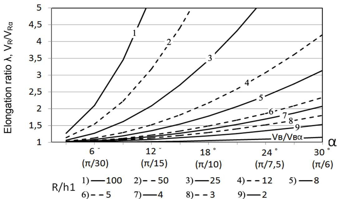
**Figure 2.** Dependence of elongation ratio  $\lambda$  and ratio  $V_R/V_{R\alpha}$  on rolling parameters. Area of high elongation ratios ( $\lambda \leq 5$ )
