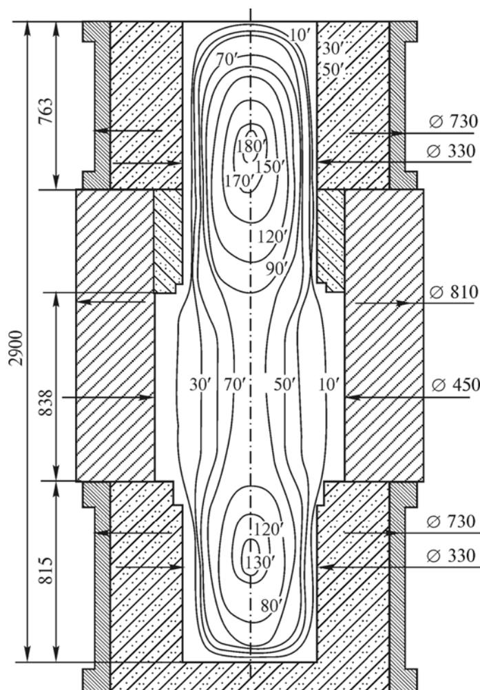
**Figure 2.** Calculated curves of solidification front isosolidus in cast iron roll with spheroidal graphite at pouring temperature 1320 °C: 10', 30', 50', 70', 80', 90', 120', 130', 150', 170', 180' - time, min
