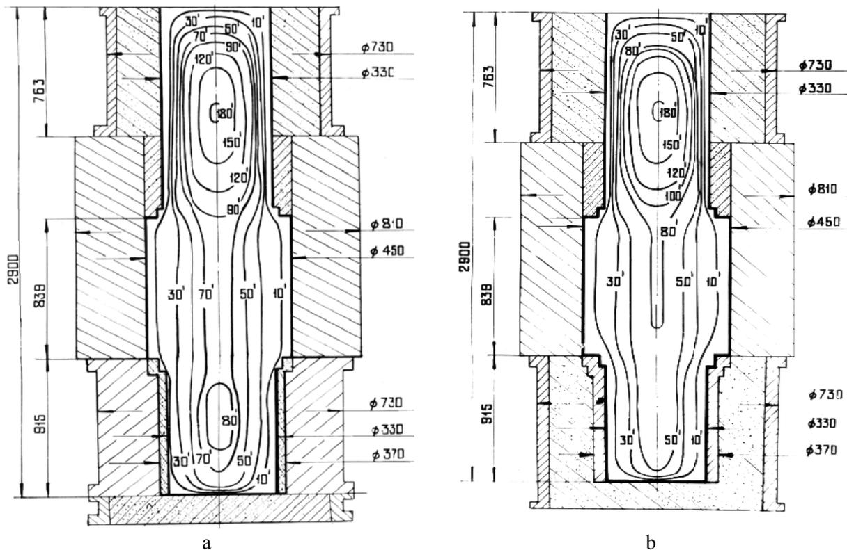
**Figure 3.** Calculated curves of solidification front isosolidus in cast iron roll with spheroidal graphite at pouring temperature 1320 °C: *a* – bottom neck is produced in the chill mold with sand- argillaceous heat insulation 20 mm thick; *b* - bottom neck is produced from external steel chill 20 mm thick in the molding box with a sandy mix; 10', 30', 50', 70', 80', 90', 100', 120', 130', 150', 170', 180' — time, min
