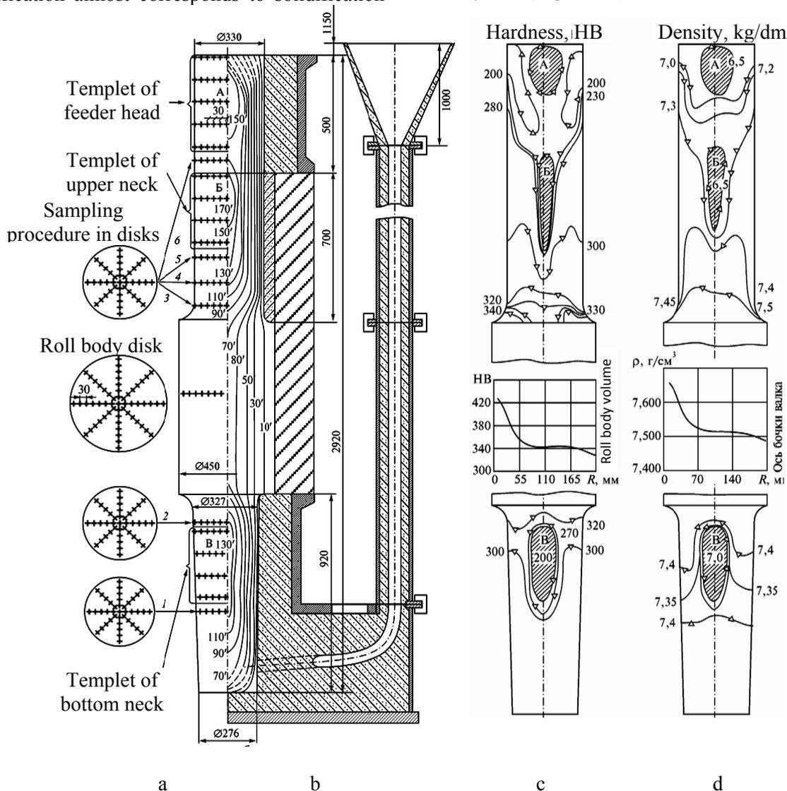
**Figure 1.** Template and disk cutting, sample taking (a) from 2200 kg roll made of cast iron with spheroidal graphite, isosolidus front at solidification and mold (b), change of hardness (c) and density (d) across the thickness and height of the cast
