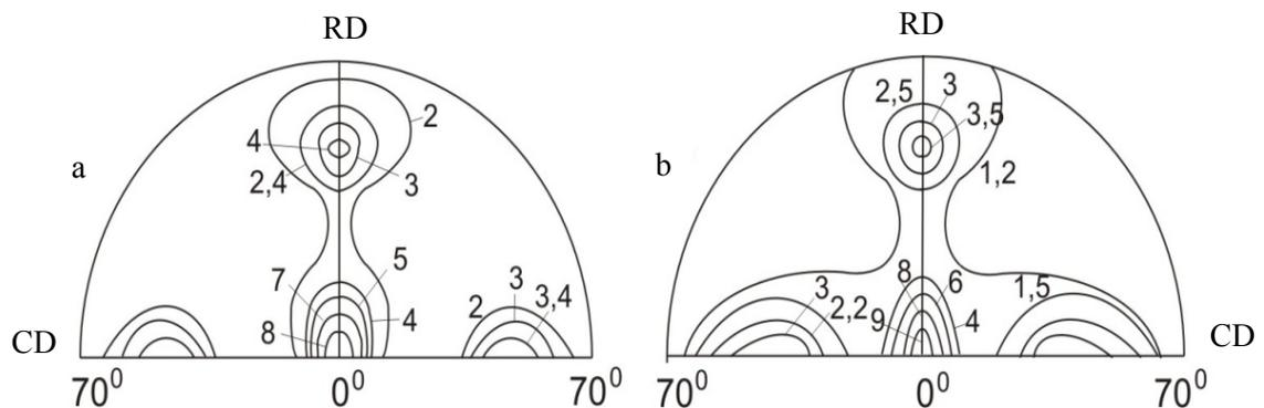
**Figure 1.** Pole figures (0002) of AZ31 sheets after deformation: *a* - 1 cycle; *b* - 8 cycles of sign-variable bending
