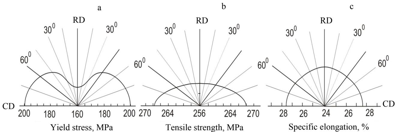
**Figure 2.** Anisotropy of yield stress (a), tensile strength (b), specific elongation (c) of AZ31 sheets after hot rolling and recrystallization annealing
