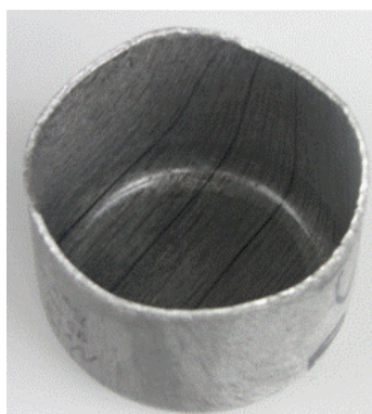
Figure 7. Cup processed by deep drawing of an initially cast strip of the alloy EN AW-6082
