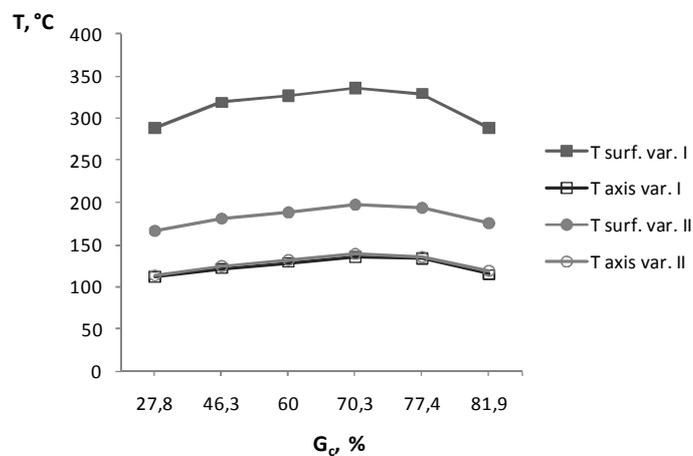
**Figure 5.** The change of temperature for wire surface and for wire axis for wires drawn in conventional way (variant I) and with use of pressure dies (variant II) in total reduction function
