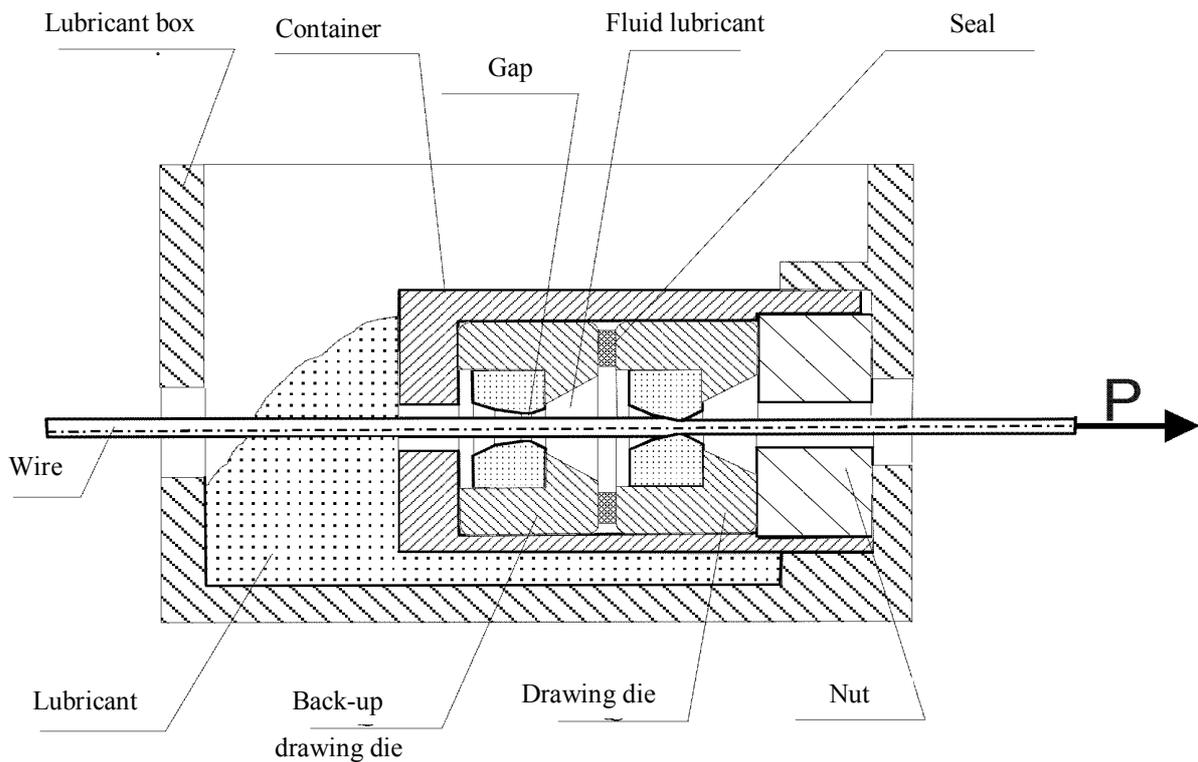
**Figure 1.** Construction and the scheme of drawing process with use the pressure die [5]
