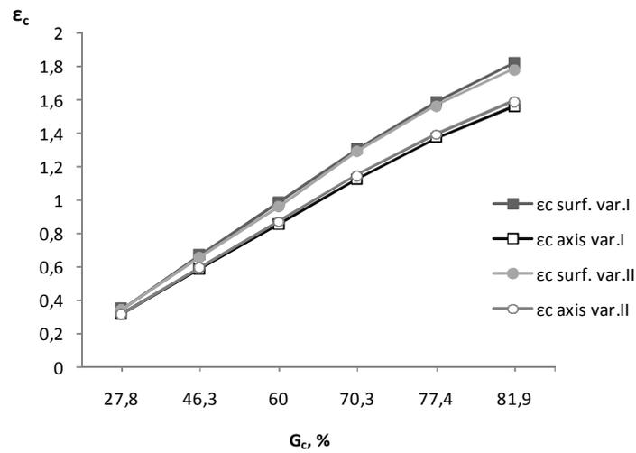
**Figure 4.** The change of strain intensity on wire surface and on wire axis for wires drawn in conventional way (variant I) and with use of pressure dies (variant II) in total reduction function
