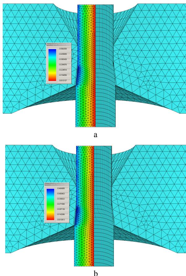
**Figure 2.** The distribution of redundant strain  $\epsilon_{xy}$  for wires drawn from diameter 1.90 mm on diameter 1.70 mm: *a* – variant I; *b* – variant II
