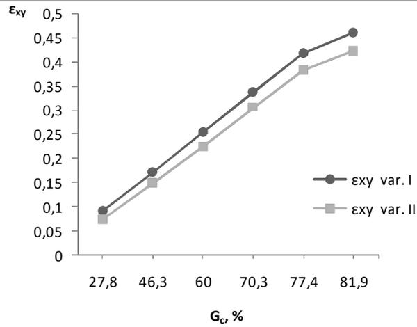
**Figure 3.** The change of redundant strain  $\epsilon_{xy}$  for wire surface drawn in conventional way (variant I) and with use of pressure dies (variant II) in total reduction function
