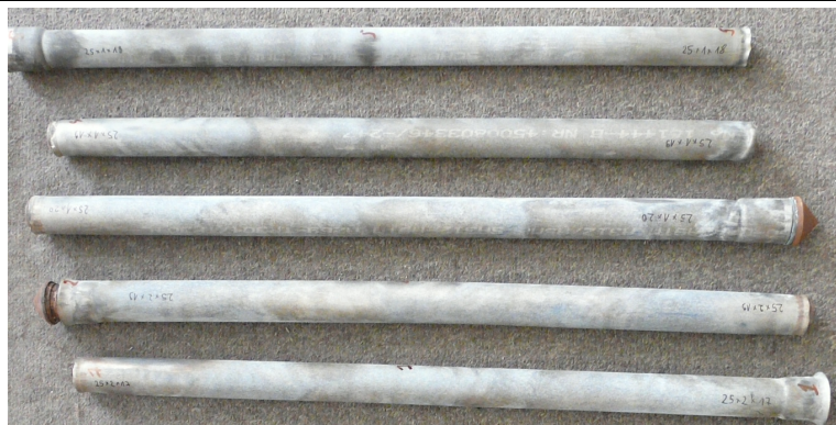
Figure 3. Bimetallic bars after explosive welding
