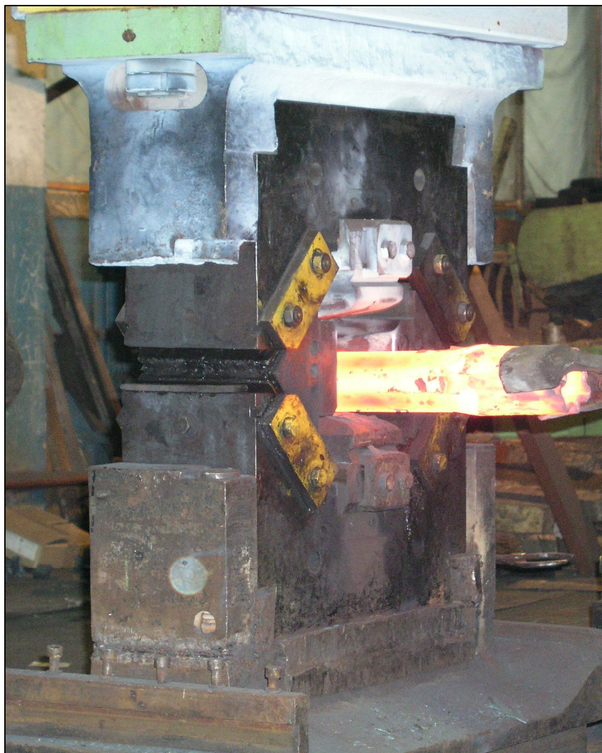
Figure 4. 4-die forging device installed in a hydraulic forging press AKII-500 SE "USSI"
