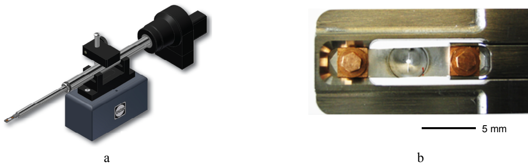
Figure 1. The Gatan 654 straining holder used for the in situ TEM tests: a – general view; b – holder with the specimen
