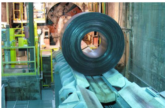
Figure 5. Material: Alform 1100 (Hot yield stress up to 1300 \text{ N/mm}^2 . Thickness – 8 mm. Coiling temperature app. 115^\circ\text{C} )
