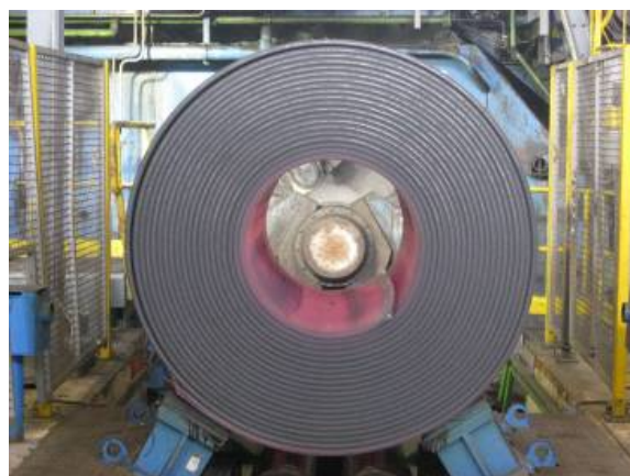
Figure 9. Material: X80 (Thickness – app. 25 mm. Width app. 1900 mm)
