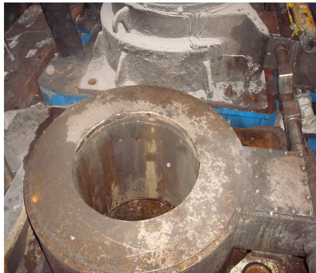
Figure 1. Six-groove CCM mold 6-strand, equipped with the EMS
