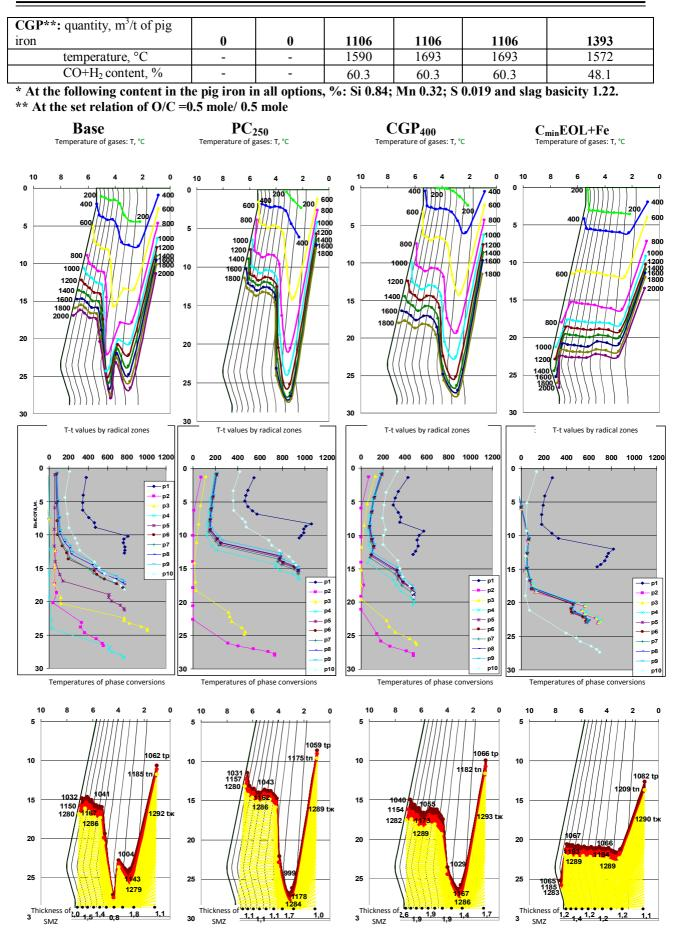
**Figure 1.** The isolines of the gas temperature (T), the temperature differences between the gas and the charge (T-t), and the parameters of the softening and melting zone (SMZ) in the workspace of BF in the base period, with pulverized coal injection, injection CGP and  $C_{min}EOL+Fe$ ; horizontal: the distance from the axis of the BF, vertical: the distance from the "technological zero" m. Initial softening point is  $t_p$ , melting point is  $t_n$ , liquid-phase flow -  $t_{xx}$
