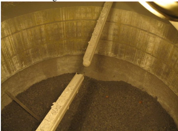
Figure 4. Influence of the thermal probe on the formation circumferential irregularity of the surface of the grist charge (surface of charge grist after unloading portion № 104, the level of the grist 4.1-4.4 m)
