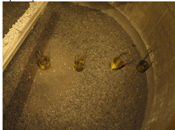
Figure 5. Installation of cylindrical samplers on the surface of coke before unloading iron ore research portion АОIII 9-4 (№ 1 - axis; № 4 - wall)
