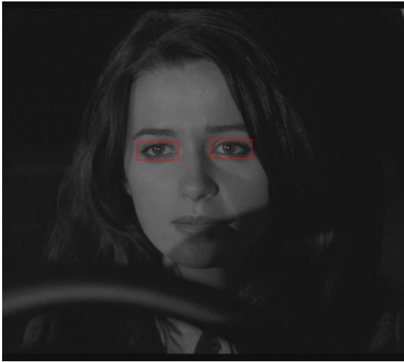
Figure 5. Improved algorithm of driver eye detection positioning results
