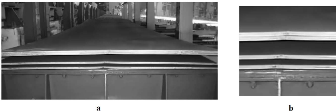
Figure 1. View of the sheets end face sheared by chevron type knives: a - general view; b - in the linkage region of the chevron knife edges
