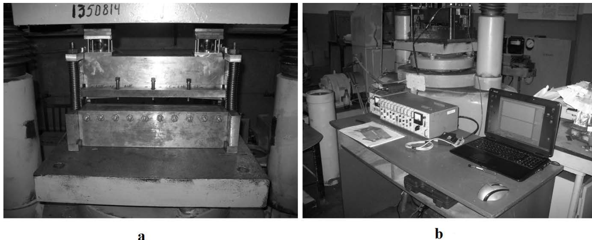
Figure 2. General view press shear installed on the press (a) and attached to the measuring system (b)
