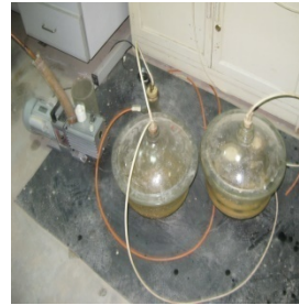
(b) Air exhaust and water saturation
