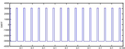
g) Comparison between inverter voltage and drive pulse under two-state hysteresis control
