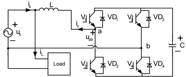
Figure 4. Structure of single-phase full bridge inverter
