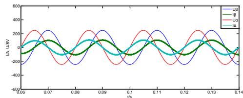
a) Output voltage, current of scott transformer under two-state hysteresis control
