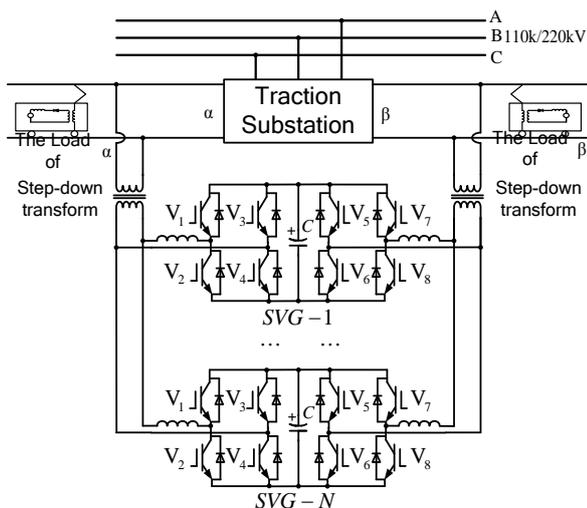
Figure 1. Compensation theory of parallel SVG with N modules
