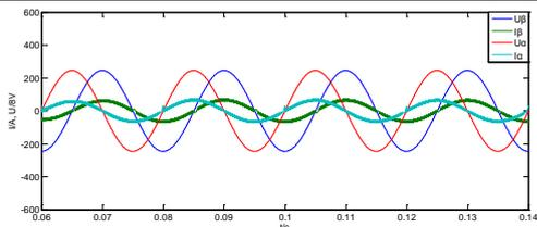
b) Output voltage, current of scott transformer under three-state hysteresis control
