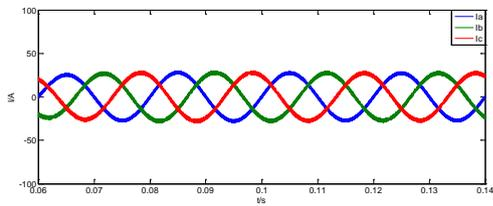
c) Three-phase current on the power grid side under two-state hysteresis control
