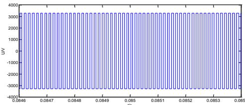
e) Inverter voltage  $u_{ab}$  under two-state hysteresis control
