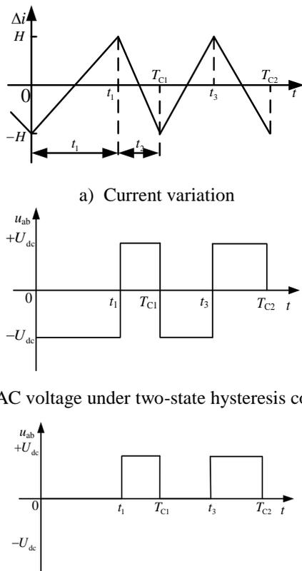
Figure 3. Schematic diagram of hysteresis control ( $i_c > 0$ )
