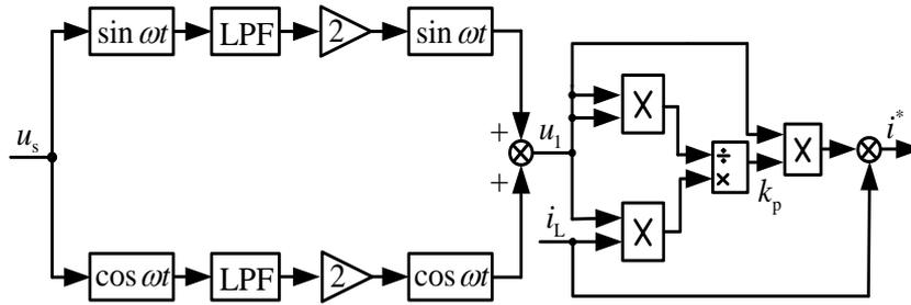
Figure 2. Schematic diagram of the single-phase synchronous detection method
