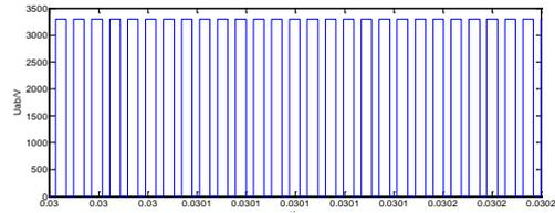
h) Comparison between inverter voltage and drive pulse under three-state hysteresis control
