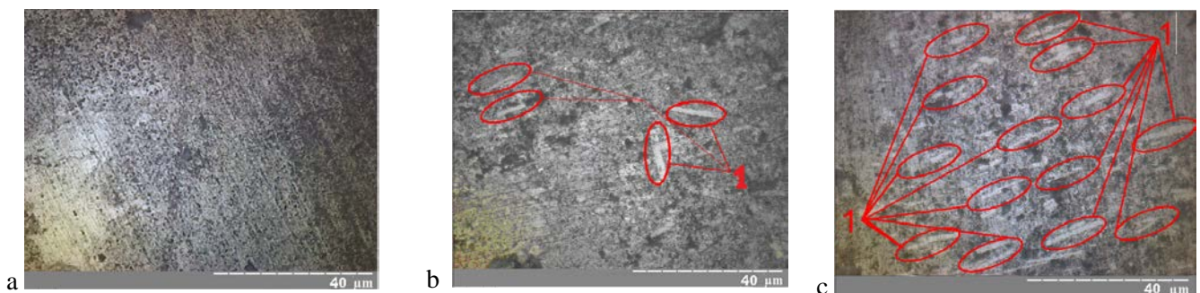
Figure 1. Photo of granite samples: a - before magnetic-hydrocavitation load; b - after hydrocavitation load; c - after magnetic-hydrocavitation load
