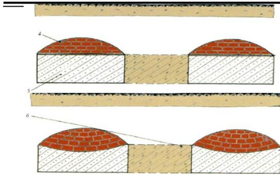
**Figure 1.** Duties of the concrete blocks by different rigidity of rocks: 1-capping material; 2-soft sediments border; 3- top formation; 4- structure blocks of rocks; 5- soft self-hardening mixtures; 6- hard self-hardening mixtures; H – operating depth, m; h – natural balance arch height.
