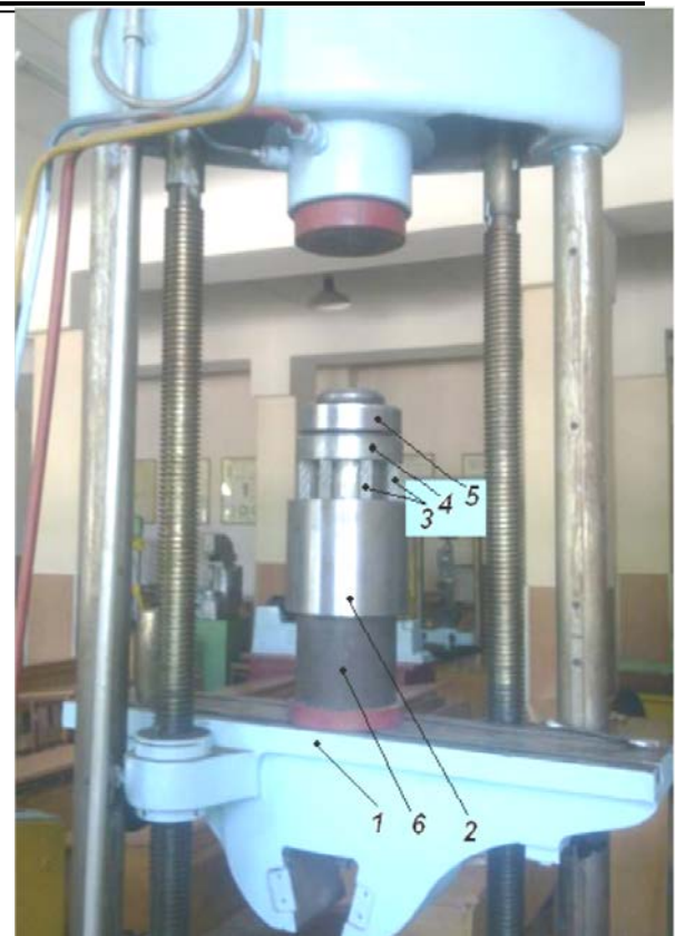
Figure 3. Segment of installation of cable LOD on universal testing machine HMS-20 before compression (break-in) of cable-elastic damping inserts: 1 – machine frame; 2 – body of cable LOD; 3 – cable inserts; 4 – upper separator; 5 – laboratory equivalent of the rod-pulling of the pulley block of rotary drilling rig “Ferdinand”; 6 – pipe – stand out for damper rod 5
