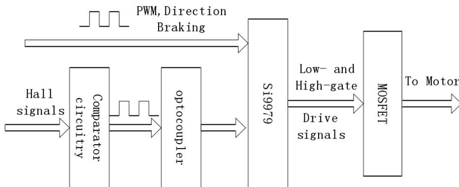
**Figure 2.** The functionality of Si9979 circuitry
