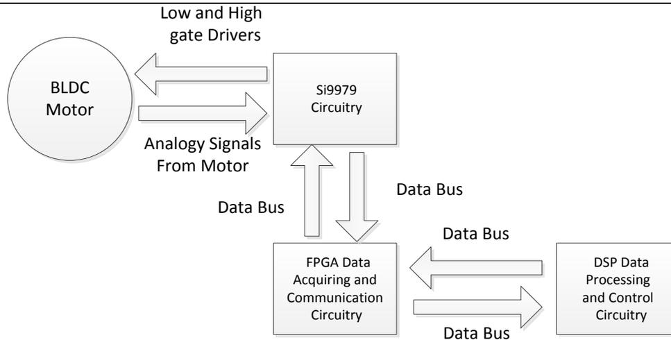
**Figure 1.** The frame of BLDC motor's driving system
