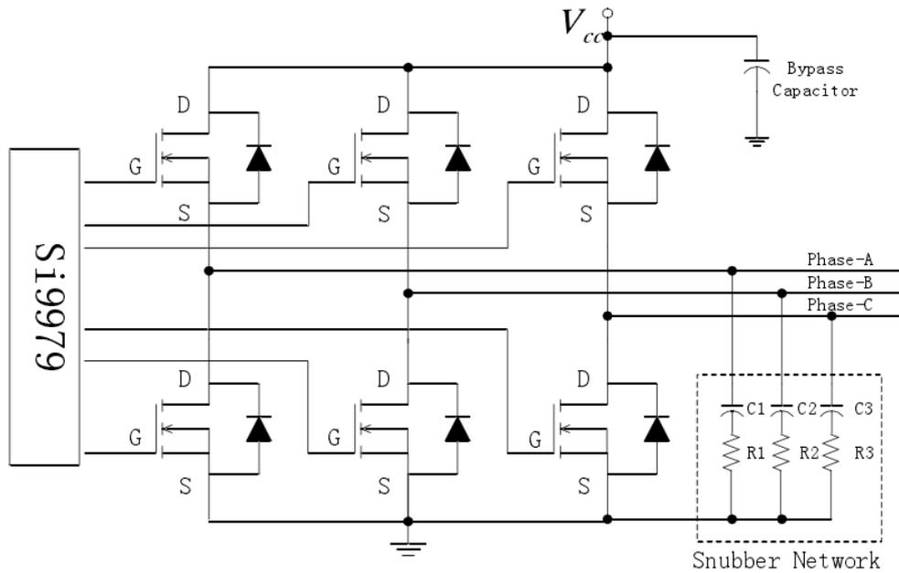
Figure 3. The power electronics with snubber network
