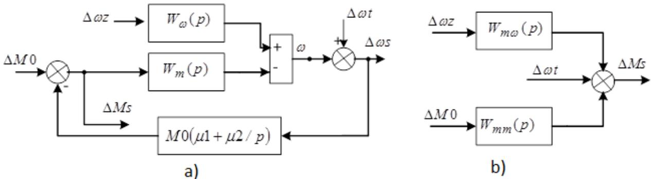
**Figure 1.** The structural diagram of speed stabilization system in free-rolling mode
