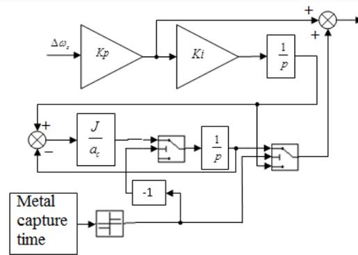
Figure 2. The speed controller with varying structure
