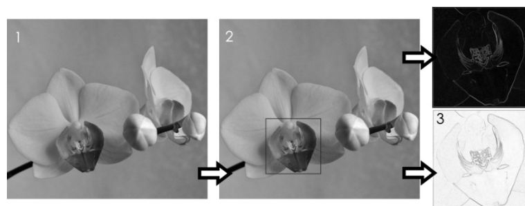
Figure 1. Process of creation of a template for further identification of object: 1 – the combined IR picture using compression of the grayscale image; 2 – application of the Viola-Jones method; 3 – the Sobel operator in normal and inverse options
