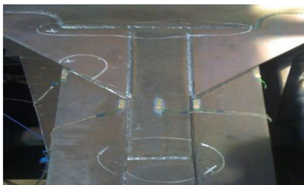
The Crack in the Drawbar of the Long Wheelbase Flat Wagon
