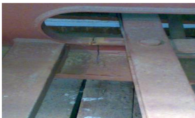
The Crack in the Backframe of the Long Wheelbase Flat Wagon
