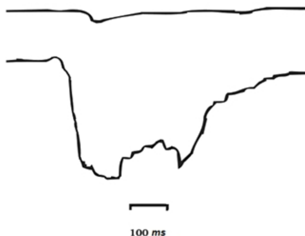
Figure 3. The oscillograms, fixing process of deformation of the tubular shock-tube: 1 - when the action of the shock wave; 2 - when the action of the detonation wave
