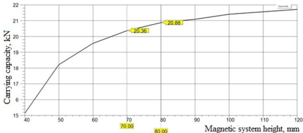
**Figure 4.** Dependence of carrying capacity on height of magnetic system with diameter of 150 mm
