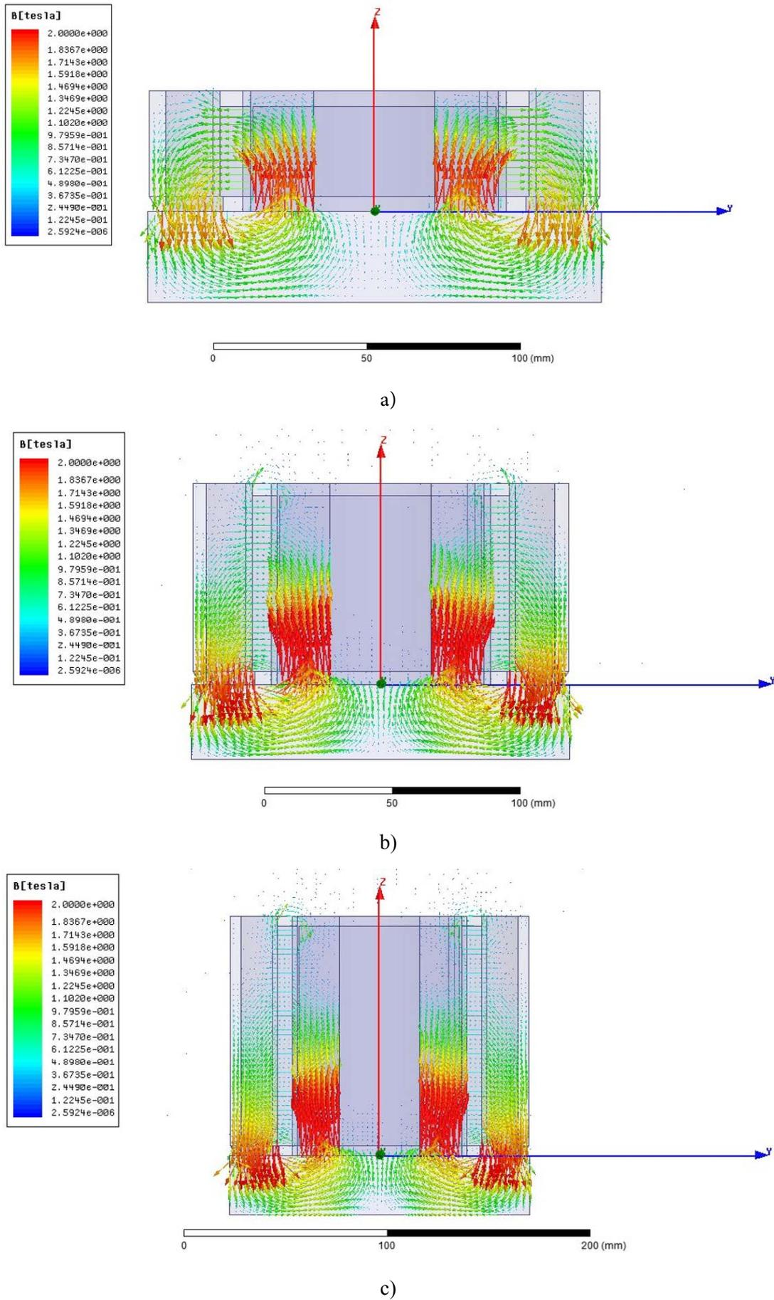
**Figure 5.** Vector graphics of magnetic induction distribution of systems of 40 mm (a), 80 mm (b), 120 mm (c) in height
