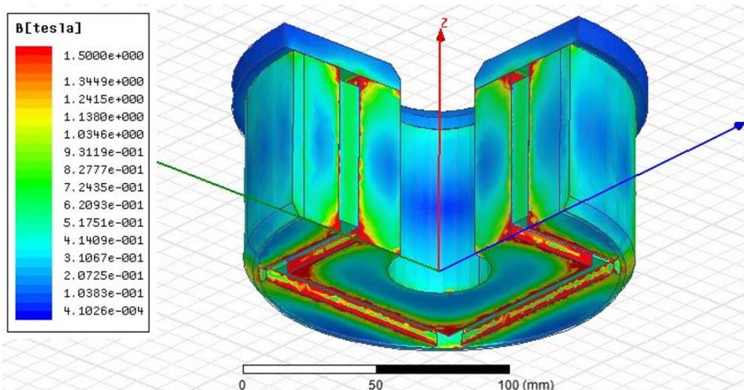
**Figure 6.** Distribution of magnetic induction in system without ferromagnetic plate
