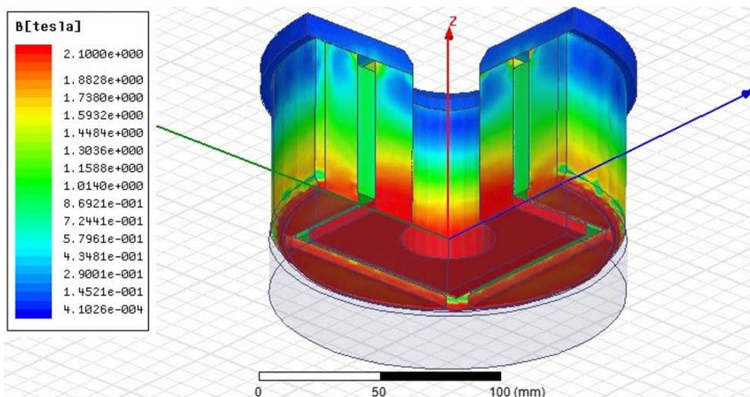
**Figure 7.** Distribution of magnetic induction in system with ferromagnetic plate
