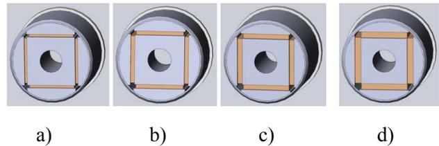
**Figure 2.** Models of magnetic systems with diameter of 150 mm with a length of magnets of 6 mm (a), 8 mm (b), 10 mm (c) and 12 mm (d)
