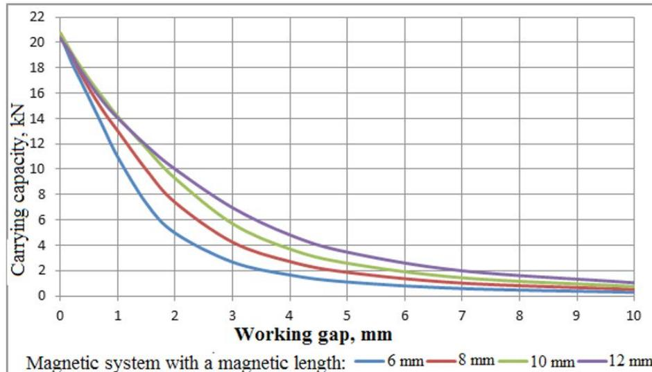
**Figure 3.** Traction characteristics of systems with a diameter 150 mm with magnets of different length
