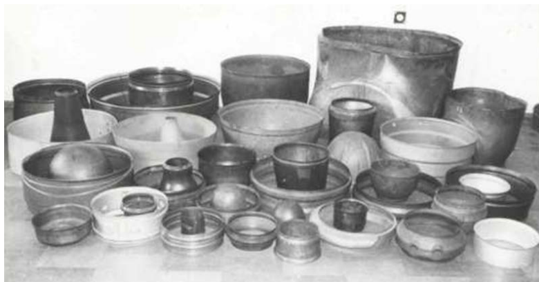
Figure 1. General view of the parts produced by explosive stamping of welded cylindrical blanks
