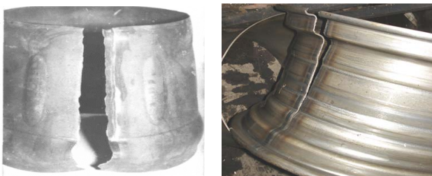
Figure 3. Types of destruction of welded cylindrical blank in the weld zone during forming
