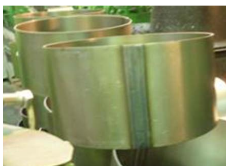
Figure 4. Type of the blank with weld seam prior to profiling of the wheel rim
