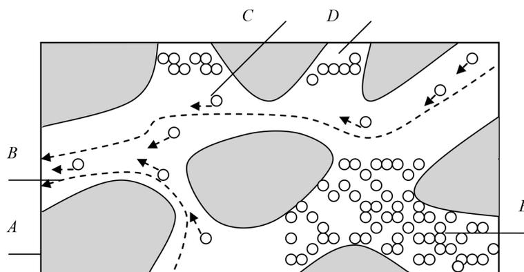
**Figure 1.** The scheme of the filtration efficiency of the porous permeable materials of saponite - titanium system composite:  $A$  - porous permeable medium;  $B$  - water movement;  $C$  - particles release;  $D$  - water associated with the precipitate;  $E$  - precipitate
