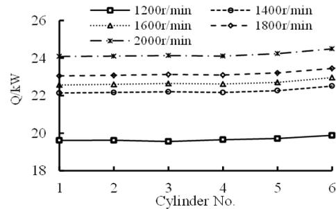
**Figure 6.** Heat Transferred From Combustion Gas to the Engine Body
