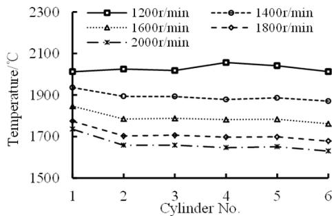
(a) Maximum Temperature of the Combustion Gas in the Cylinder
