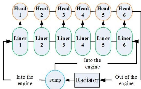
**Figure 3.** Cooling Water Flow in the Engine
