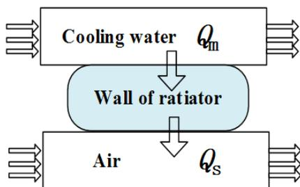
**Figure 2.** Heat Transfer of the Radiator
