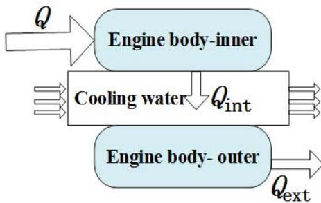
**Figure 1.** Thermal Balance in Cylinder
