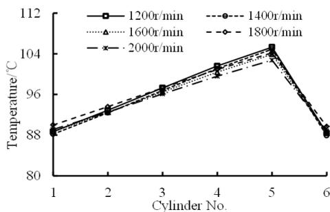
(b) On the Surface of Cylinder Liners
