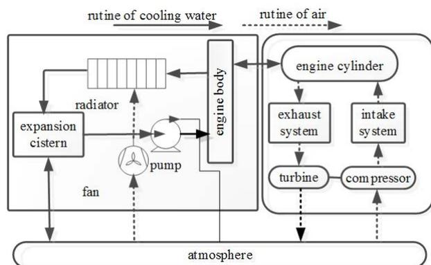
**Figure 4.** Diesel Engine Working Process Simulation Model Coupled With Cooling System
