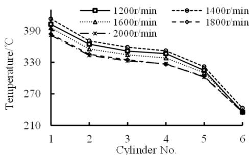
(c) Maximum Surface Temperature of the Cylinder Head
