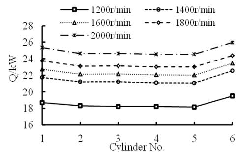
**Figure 7.** Heat Transferred to the Cooling Water From the Engine Body
