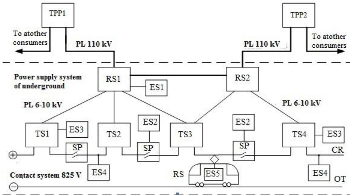
**Figure 1.** Structure scheme of the underground power supply system with possible placements of energy storages
