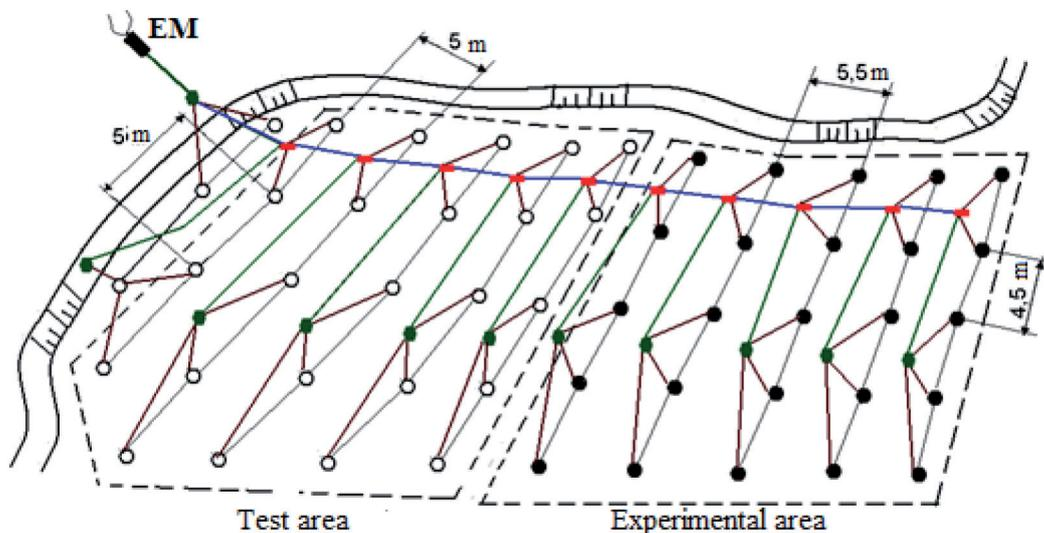
**Figure 2.** The diagram of placement of boreholes and charges commutation in pit shoulders of “Zvirky”, unit 46, mount. – 42.0 m
