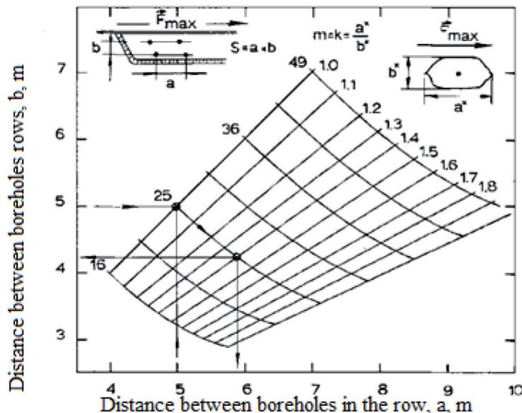
**Figure 1.** The nomogram for correction of boreholes considering anisotropy coefficient
