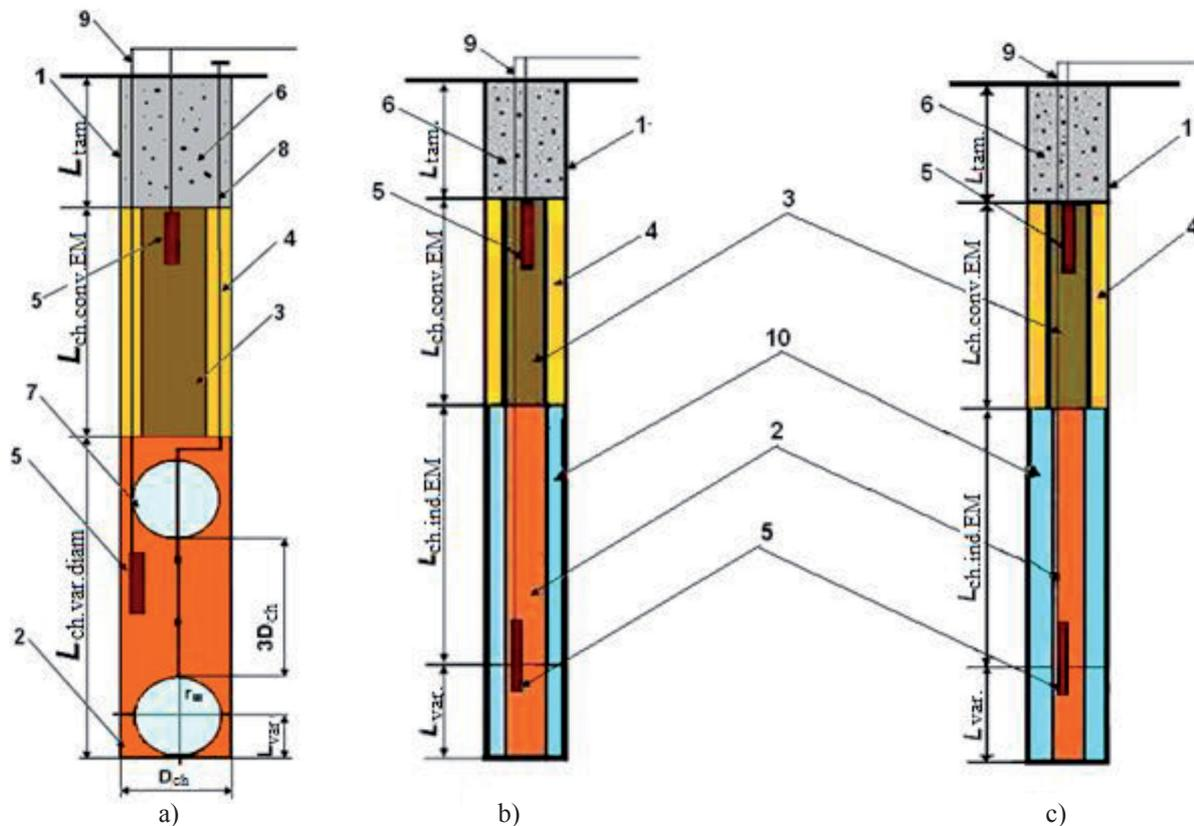
**Figure 3.** Structure of the borehole multicharges: a) variable diameter; b) charge in square prism section; c) charge in triangular prism section; 1 – borehole; 2 – charge of mixed EM – HG + AN; 3 – section of conversion EM - DKRP-4; 4 – pyroxylin powder; 5 – primed blasting cartridge; 6 – tamping; 7 – spherical cavities; 8 – binder for connection of spherical cavities; 9 – non-electric system of initiation «Impuls»; 10 – inert interval
