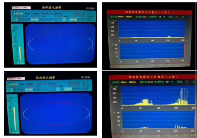
Figure 5. Point Discharge PD Pulse Map under the Voltage (3.5kV VS. 4.5kV)
