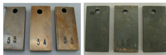
Figure 4.1. The macro morphology of B30 after comprehensive corrosion (a)contained no \text{H}_2\text{S} (b)contained \text{H}_2\text{S}=2000\text{mg/L}
