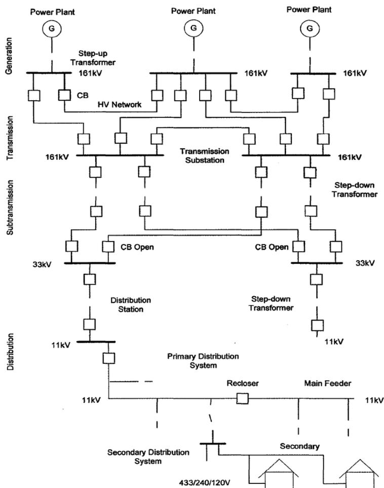
**Figure 1.** A basic model of power supply system
