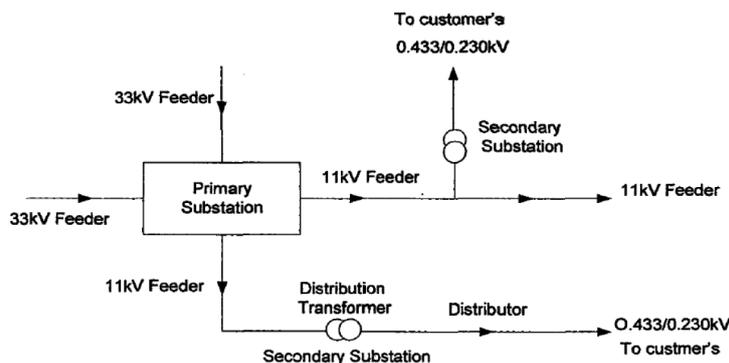
Figure 2. The radial distribution network
