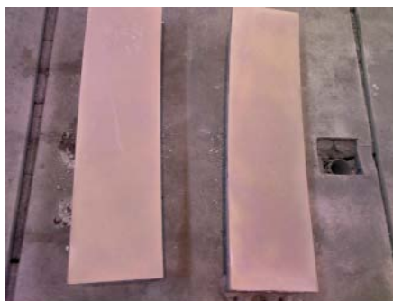
Figure 2. The walls of the mold after the heat treatment in a shielding atmosphere (H 2 ) at 900 ° C for 10 hours
