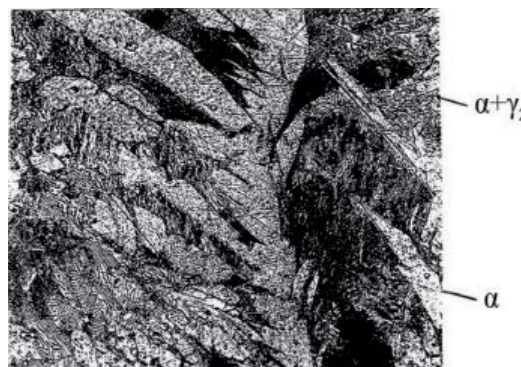
Figure 1. The microstructure of diffusion layer (sample No 1), \times 500
