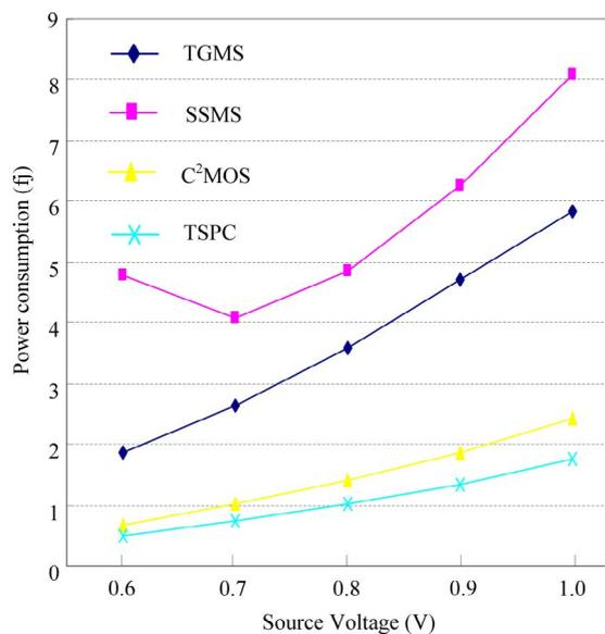
Figure 12. Power consumption of four flip-flops
