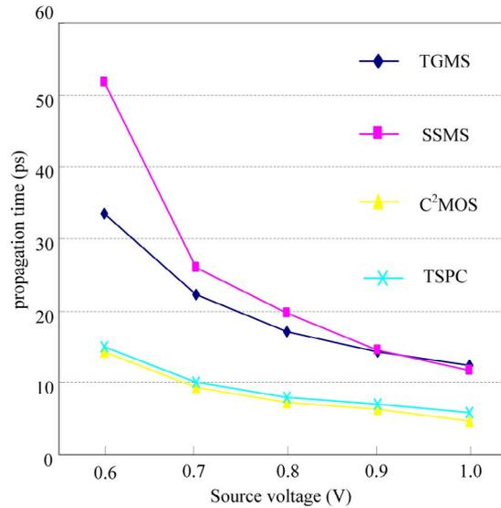
Figure 11. Propagation delay of four flip-flops
