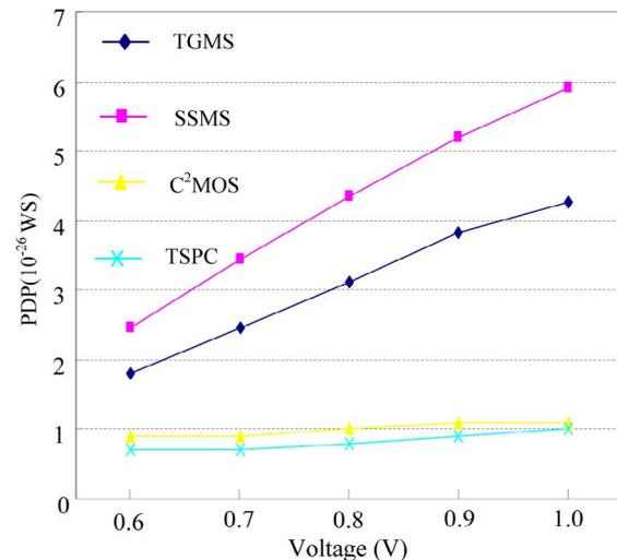
Figure 13. PDP of four flip-flops
