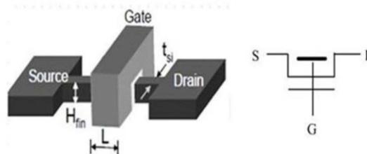
**Figure 1.** The structure and symbol of FinFET
