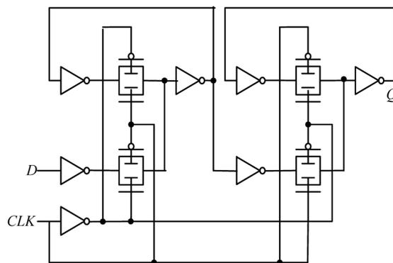
Figure 6. Transmission-gate master-slave flip-flop (TGMS)
