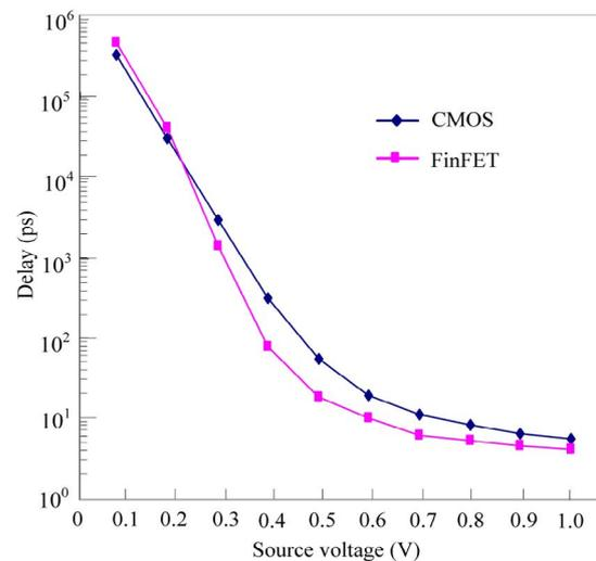
Figure 3. Propagation delay of the 32nm FinFET and bulk CMOS inverters
