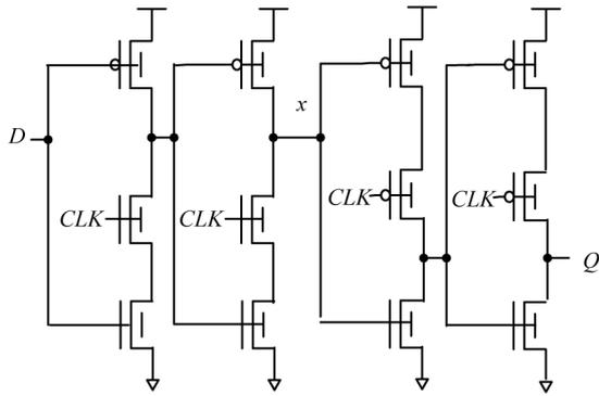
Figure 9. True single phase clock master-slave flip-flop (TSPC)
