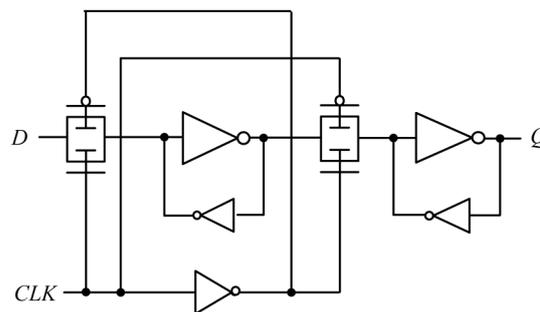
Figure 7. Simplified static master-slave flip-flop (SSMS)
