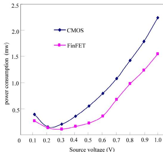
Figure 4. Power consumption of the 32nm FinFET and bulk CMOS inverters
