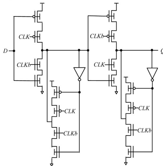
Figure 8. Clocked CMOS Master-Slave flip-flop ( $C^2$ MOS)
