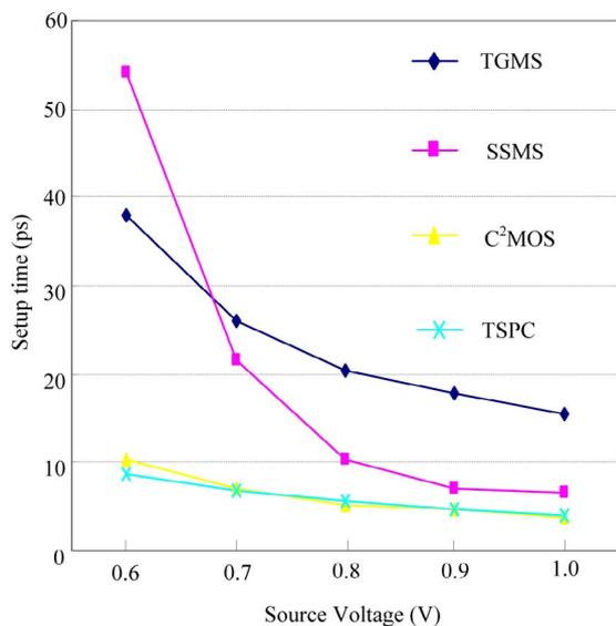
Figure 10. Setup time of four flip-flops
