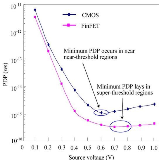
Figure 5. PDP of the 32nm FinFET and bulk CMOS inverters
