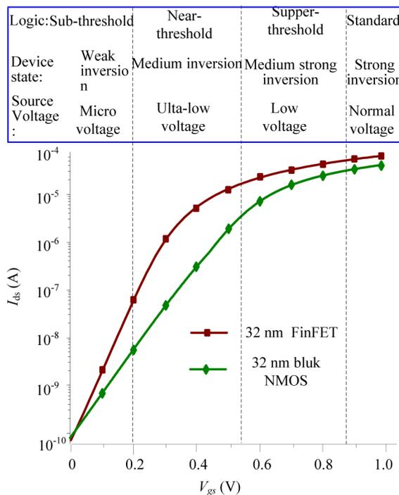
**Figure 2.** I-V characteristics of 32 nm n-type FinFET and conventional bulk NMOS transistor
