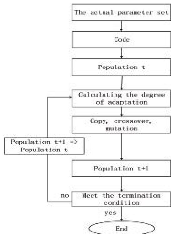
Figure 3. Genetic algorithm basic flow chart
