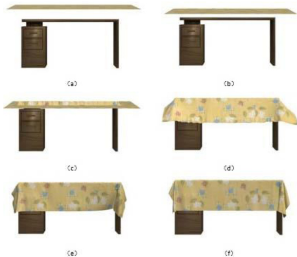
Figure 8. Effect picture of simulation through the application of Velocity-Verlet integration algorithm
