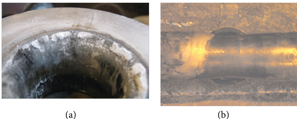
Figure 1. Wear pattern of matrix a) and mandrel b) of pipe section press.
