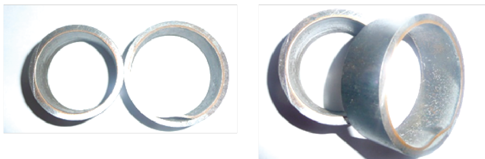
Figure 2. Templates of the pressed finished bimetallic pipes with a number of violations of a bimetallic layer.
