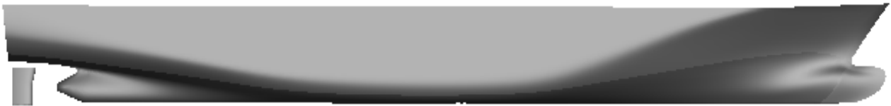
Figure 2. The 3D geometry model of hull and rudder by “Yu-Kun”
