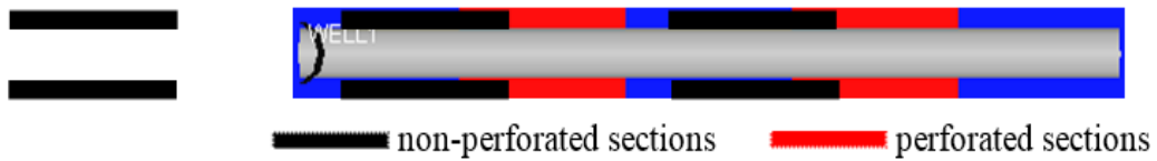
Figure 6. Synthetic well completion method
