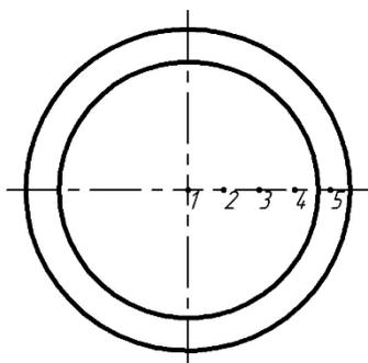
**Figure 2.** Points of testing hardness of samples
