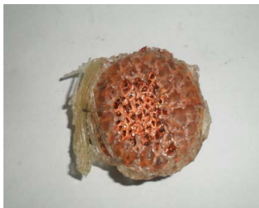
Figure 5. Diagram of the copper foam after the compression test
