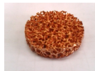
Figure 3. The copper foam used in this compression test
