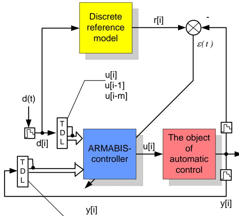
Figure 1. System architecture of model reference adaptive control
