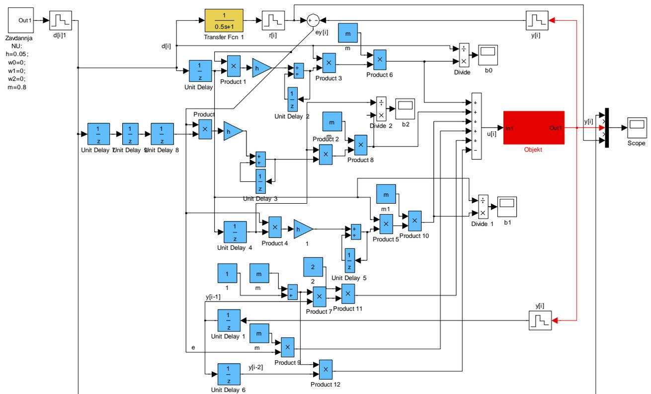
Figure 2. Matlab-model of adaptive control of non-stationary second-order object with ARMABIS-regulator and reference model
