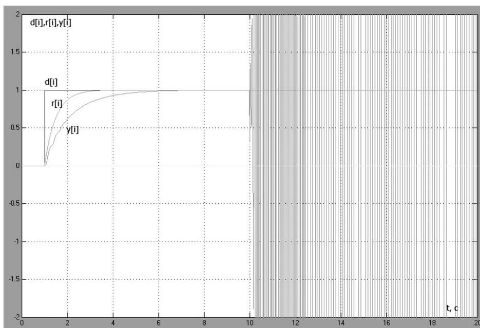
**Figure 6.** Transition processes along the output coordinate  $y[i]$  of control object, task signal  $d[i]$  and reference model  $r[i]$  at regularization coefficient of *ARMABiS*-structure  $\mu=11,5$
