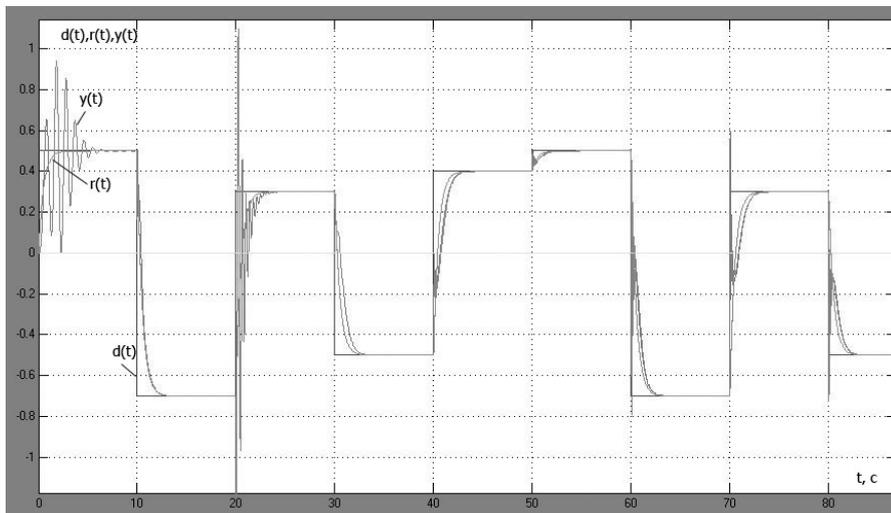
**Figure 4.** Transition processes in classic adaptive system of neurocontrol of non-stationary second-order object
