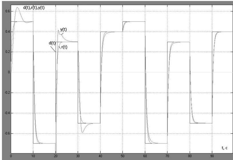
**Figure 3.** Transition process in adoptive control system with *ARMABiS* –regulator during the initial period of work (d(t) – task signal, r(t) – reference type of transition process, y(t) - isolated yield of control object)
