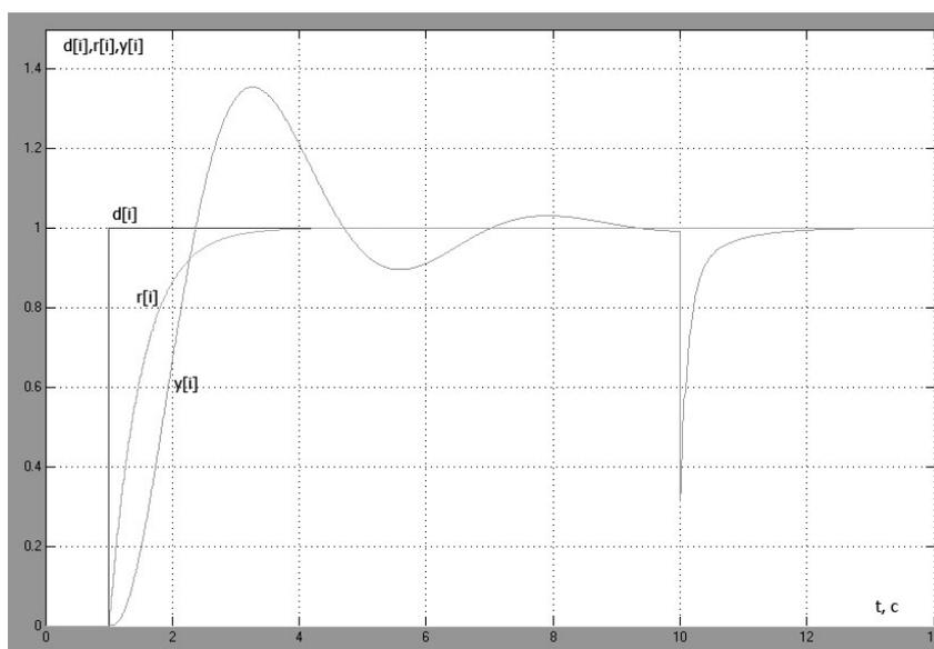
**Figure 5.** Transition processes along the output coordinate  $y[i]$  of control object, task signal  $d[i]$  and reference model  $r[i]$  at regularization coefficient of *ARMABiS*-structure  $\mu=0,8$
