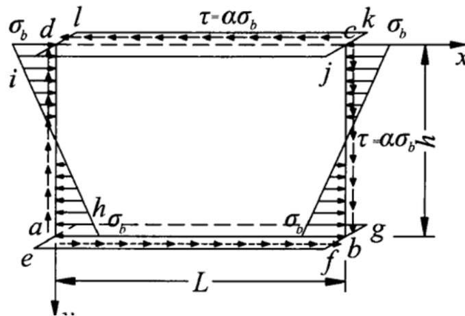
Figure 3. A schematic diagram of the web under the action of bending and shearing
