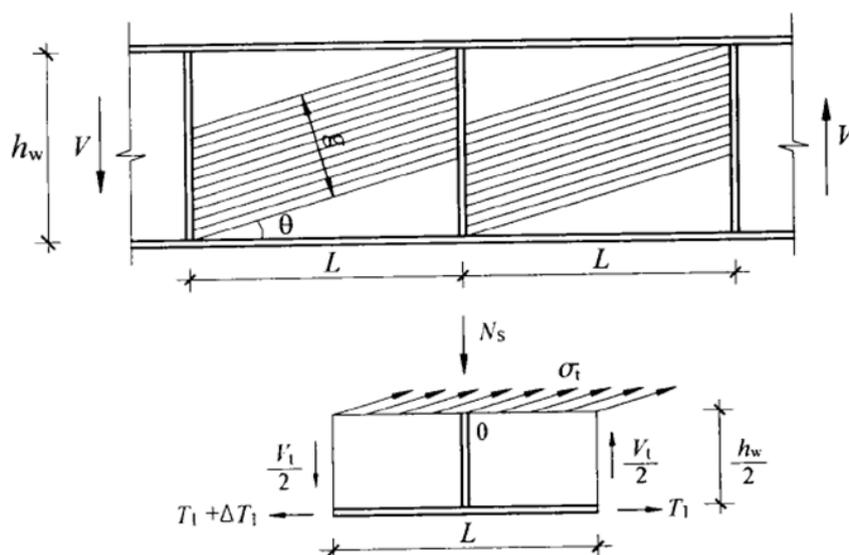
Figure 1. Computational model of Basler's theory
