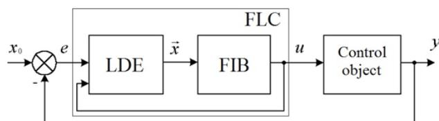
**Figure 1.** The block diagram of the fuzzy ACS over a channel “mixture ignition temperature - the temperature in the vacuum chamber 24”
