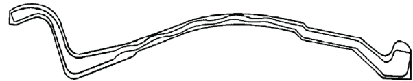
Figure 9. The rim rolling finishing and prefinishing templates with the central wavy part
